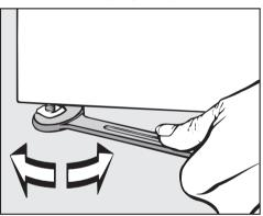
The screw feet can be adjusted to compensate for any unevenness in the floor.
